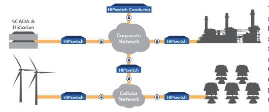
The solution provides a secure overlay network among HIPswitch™ appliances that secures remote connections for SCADA systems and remote access users. The HIPswitch Conductor™ orchestration engine coordinates configuration, security policies, trust relationships, monitoring and analytics.
