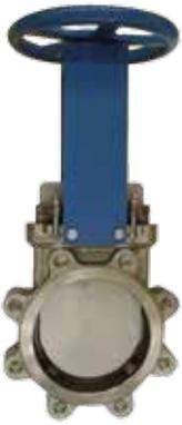
The KGN-MSU Unidirectional Cast Stainless Steel Knife Gate Valves are designed to meet MSS-SP81 and have a one-piece body with integral metal seat to meet shut-off requirements. The body and the gate are available in 304 and 316 stainless steel. The packing gland is the same material as the body and supports a variety of packing types for temperatures up to 1000°F (540°C). Valves can be mounted with a variety of accessories including cylinders with limit switches and solenoids.
