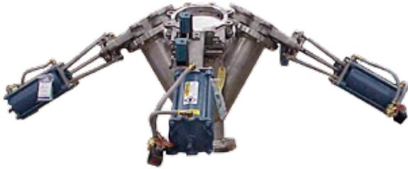
Mixing and Diverting Knife Gate Valves are available with either an integral body or a replaceable body. Valves with the replaceable body design are bolted to a Y-pattern pipe, allowing easy replacement of a single valve rather than the entire assembly.
