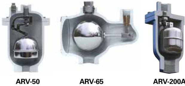
Air Release Valves function to release air pockets that collect at each high point of a pressured pipeline, and are essential for pipeline efficiency and water hammer protection. Air Release Valves are available in a wide variety of orifice sizes and materials of construction to meet a wide range of applications.
