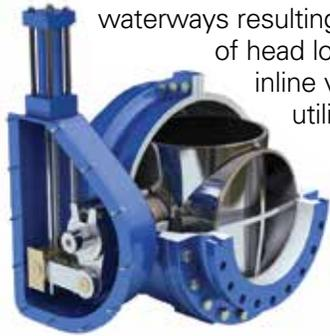
are also recommended for high velocities (above 15 FPS), flow control or buried service with critical isolation applications. Willamette AWWA Metal Seated Ball Valves are ruggedly designed with metal-to-metal seating to last for decades. Valves can be single or double seated. VBL Ball Valves can be furnished with Electric, Hydraulic or Pneumatic or Manual Handwheel operators.
