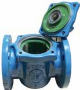
In applications where mineral build-up can be an issue, Glass Lined PEC or PEF Eccentric Plug Valves provide a smooth, non-stick glasslined interior that can inhibit crystalline formation inside the valve. Glass Lined valves are commonly used in wastewater treatment plants where Struvite (magnesium ammonium phosphate) can build up in valves, piping and equipment.
