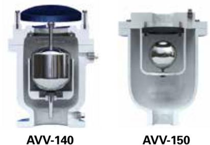
from or admitted into a pipeline as it is being filled or drained. As the pipeline fills, fluid enters the valve, raises the float and shuts-off. When draining the pipeline, the float drops and allows air to enter, preventing a vacuum and possible pipeline collapse or damaging water column separation.
