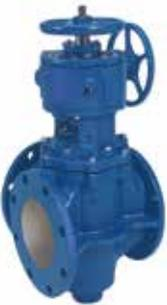
3-Way and 4-Way Plug Valves are designed for throttling and diverting of clean, dirty, viscous and corrosive liquids; sludge; abrasive and fibrous slurries; clean and dirty corrosive gases. Single and double plug styles can be arranged in a variety of flow combinations. Features include heavy-duty stainless steel bearings, long-life stem seal, resilient plug facings for dead-tight shutoff and
