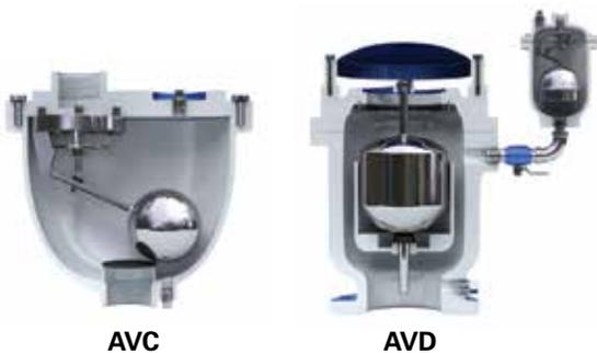
Release Valves and Air/Vacuum Valves. Combination Air Valves are installed on all high points of a system where it has been determined dual function Air Release and Air/Vacuum Valves are needed to release air and also protect the pipeline from vacuum. Combination Air Valves are available in two body styles: single body combination or dual body combination. The single body combination is used where compactness is preferred.
