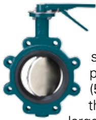
BOS-US Resilient-Seated Butterfly Valves feature an uninterrupted seat design, one-piece body, solid one-piece shaft and a high performance resilient seat. Sizes 2-20" (50-500mm) feature seat bonded to the body while sizes 24" (600mm) and larger feature a seat bonded to a solid backing ring.
