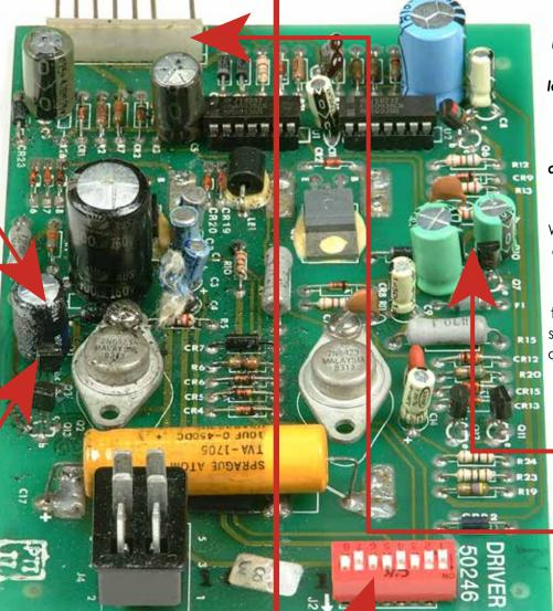
We replace and upgrade all defective low-temperature, low-quality electrolytic capacitors to 105°C. Upgrading from 85°C to 105°C more than doubles the life of your capacitors.
